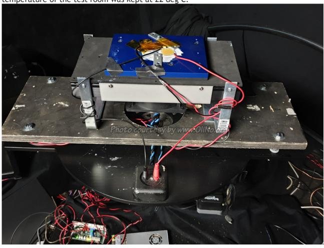
The image above shows the wooden mounting board on which the Thermo Electric Cooler is mount. The blue metal plate is the one on top of the Peltier modules. On top of this blue plate is the LED chip.
