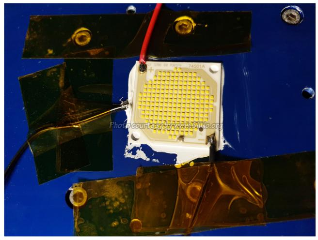
The controller has been set to maintain 25 deg C at the temperature sensor. The ambient temperature (in the test room) at 1 m distance of the test setup is controlled at 22 deg C.
