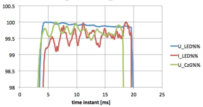
When zoomed in, we can see that the current is relatively constant at around 99.5 % of its max value. Then the voltage is slowly decreasing in value from 100 % to 99.85 % and the lux value (U\_CzG) is effectively constant over de 12 ms that the pulse is wide.
