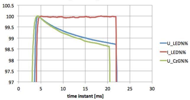
This way we can easily see (1) that both the voltage and the lux value (U\_CzG) are decreasing notably over the length of the current pulse. And (2) that the current value remains well constant. Note that for these graphs n averaging filter of 1 ms period has been used.
