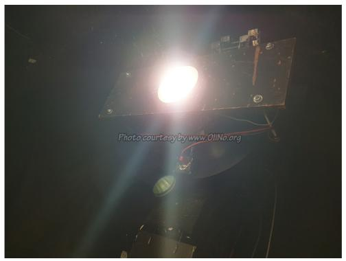
A wooden plate is used to mount the spot lamp. Then the robot is positioned to have the spot emitting light sideways.
