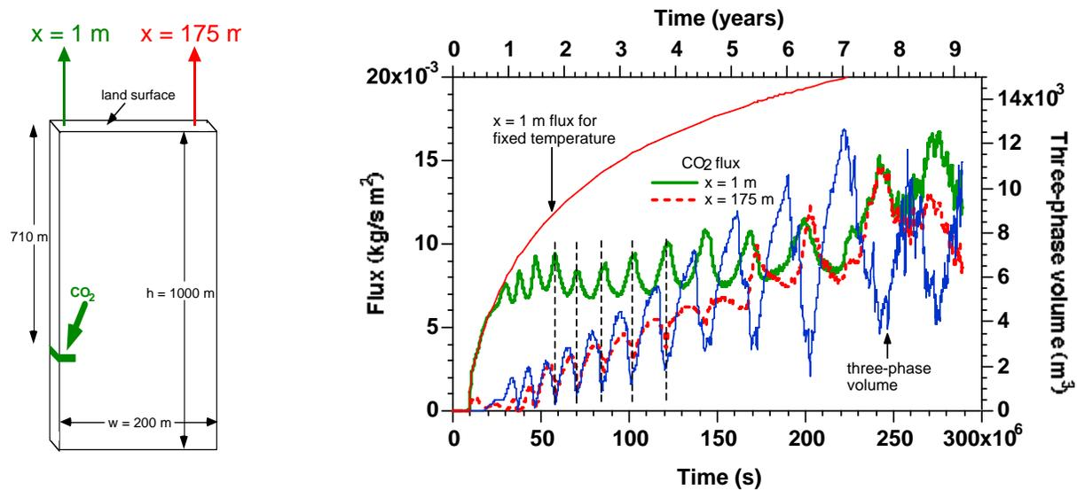
Figure 1. *CO<sub>2</sub> leakage along a fault zone (from Pruess, 2005). A schematic model of a fault zone is shown on the left. The right panel gives temporal variation of CO<sub>2</sub> leakage fluxes at two different positions at the land surface. Total flow system volume with three-phase conditions is also shown.*
