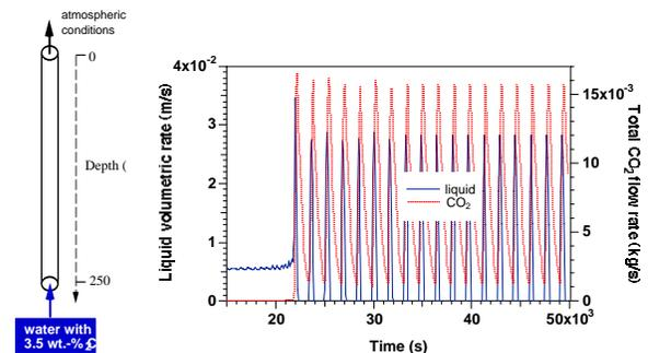
Figure 2. *Discharge of a water-CO<sub>2</sub> mixture from a well. The wellbore model is shown on the left, while the right panel shows simulated discharge rates from the well.*
