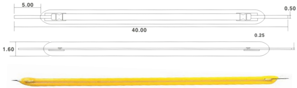
Figure 2-6. Dimensioned (mm) diagram of LED filament and close-up photograph
