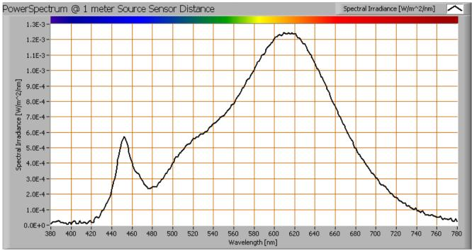
The spectral power distribution of this light bulb, energies on y-axis valid at 1 m distance.
