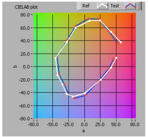
CQS-values for the light of this light bulb compared with those of a reference source with the same color temperature.
