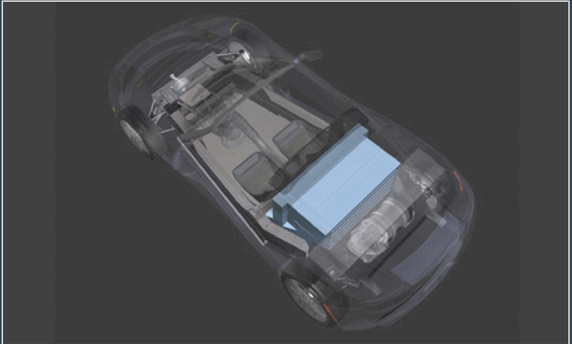
The Energy Storage System (ESS) – comprised of several thousand consumer-grade lithium-ion cells – is the heart of the Tesla Roadster. Battery conditions are continuously monitored and fed to the Vehicle Management System (VMS), allowing for precise tracking of battery history, performance, and available energy.
