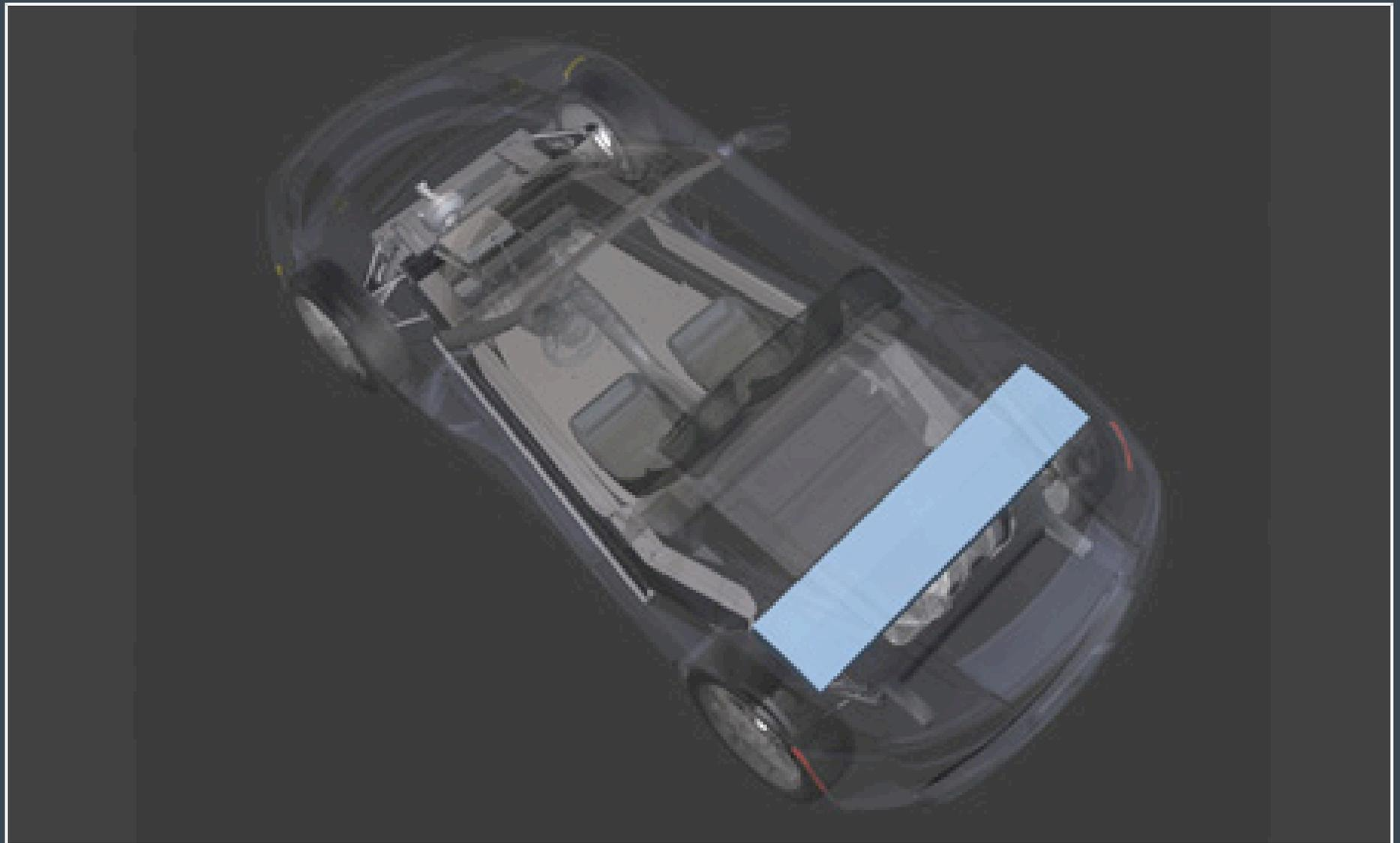
The Power Electronics Module (PEM) contains high voltage electronics that control the motor and allow for integrated battery charging. The motor and PEM have been designed as a tightly integrated system that delivers up to 185 kW of motor output.
