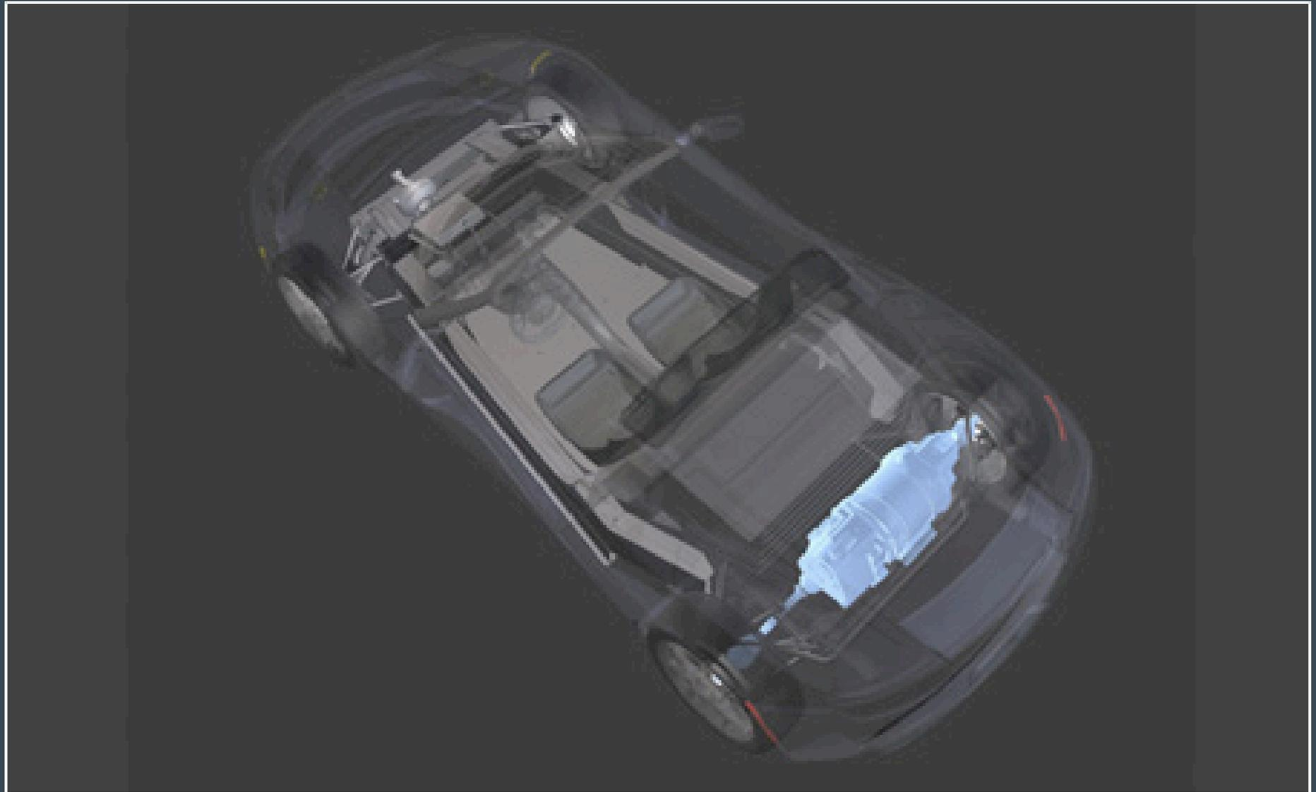
The Tesla motor weighs less than 70 pounds yet produces horsepower equivalent to a much heavier internal combustion engine. And unlike a gasoline engine, Tesla's electric motor doesn't sacrifice mileage for performance.
