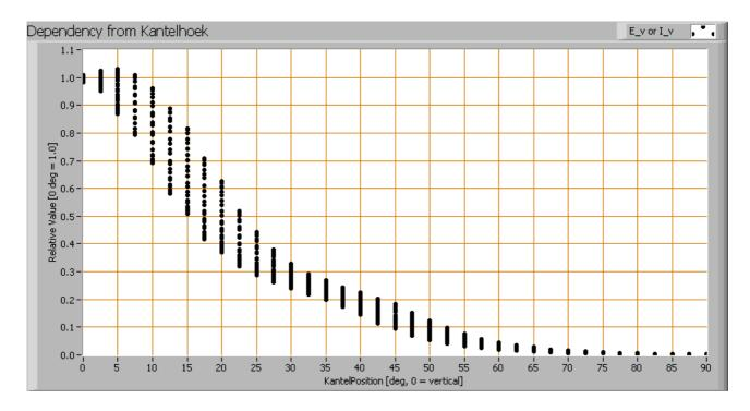
*Intensity data of every measured turn angle at each inclination angle.*
