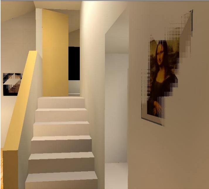
**Figure 12**      **Coplanar surface problems**
