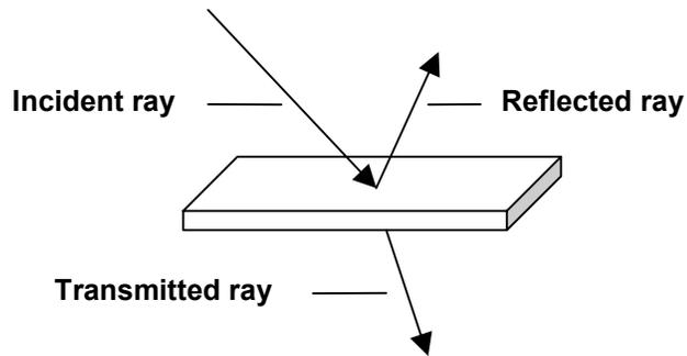
**Figure 3 BRDF / BTDF measurements**
