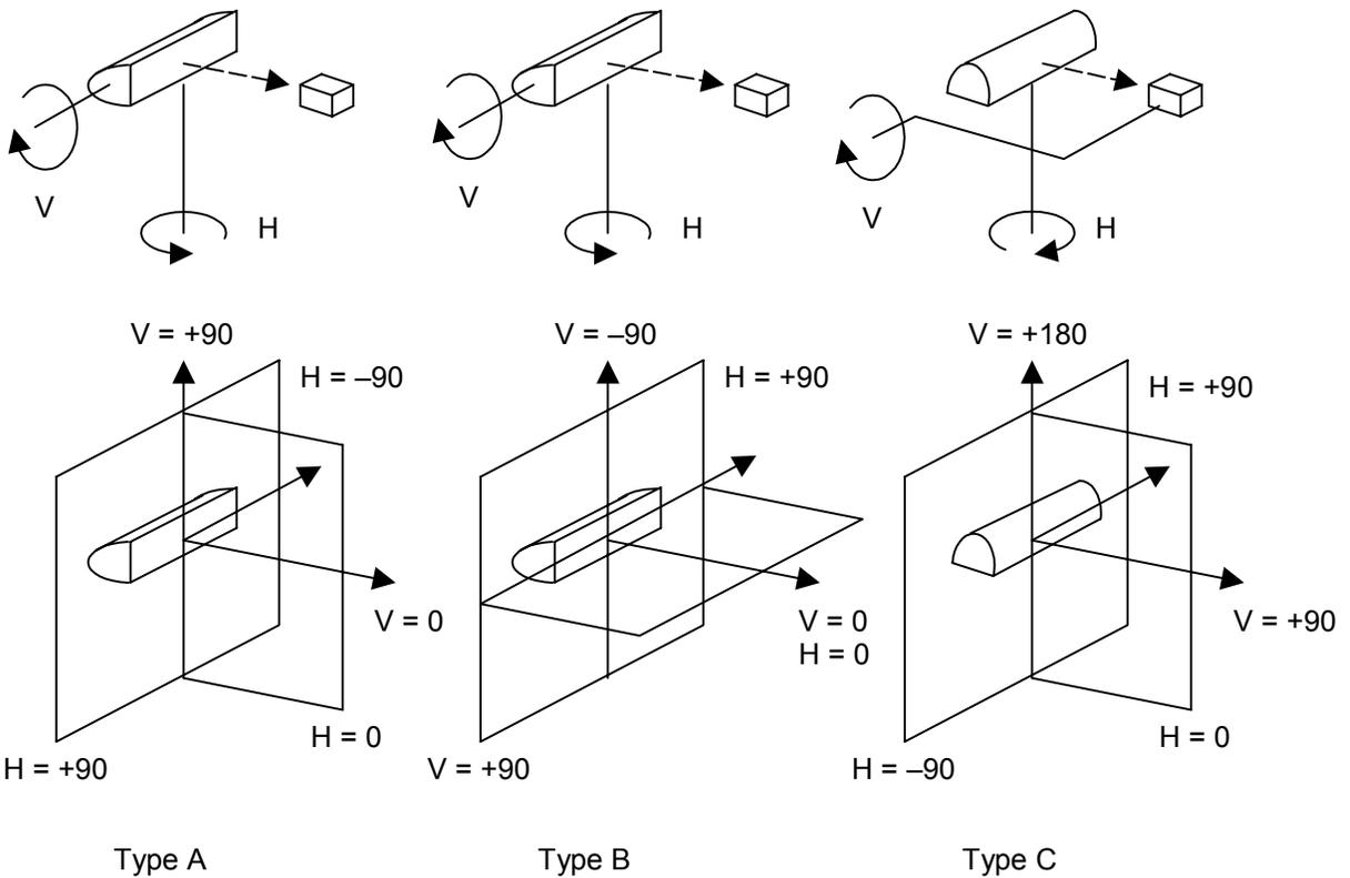
**Figure 6 Photometer Types**
