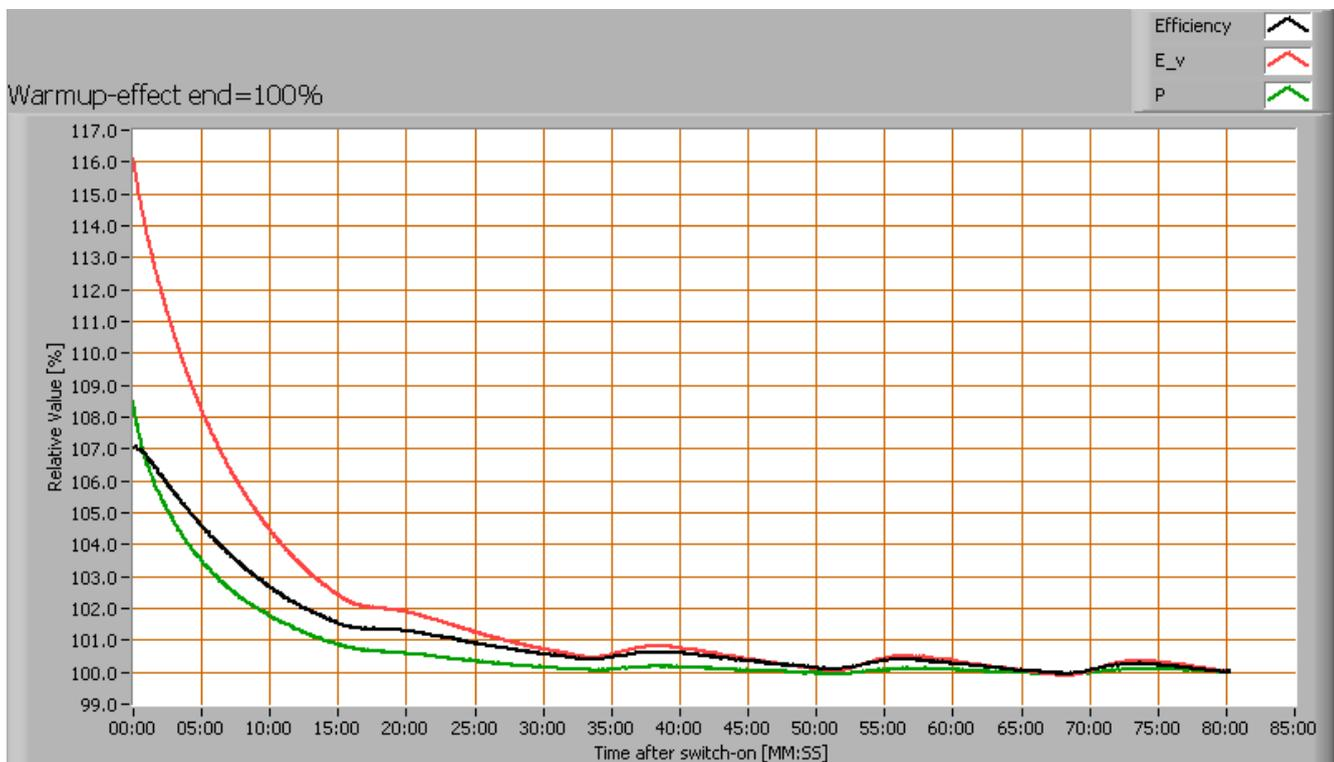
Effect of warming up on different light bulb parameters. In the first graph the 100 % level is put at begin, and in the last graph the 100 % level is put at the end.
