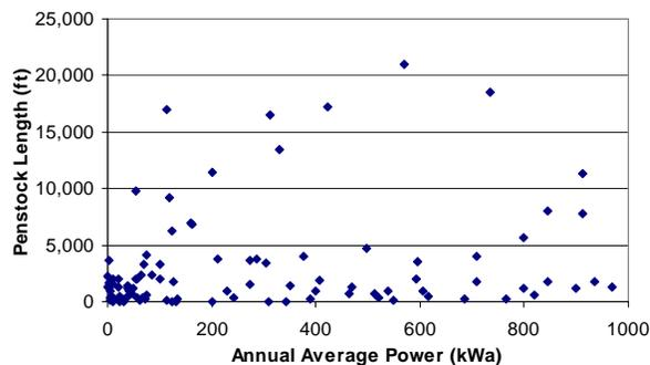
Figure 4. Penstock lengths of low power hydroelectric plants in the Pacific Northwest Region.
