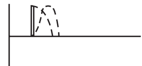
Holding current is not reached with a short driving pulse due to the delayed current
