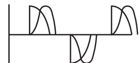
The shapes of the curves of the voltage and current with an inductive load (current is delayed)
