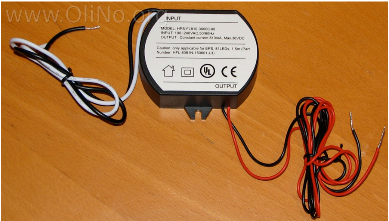
The PSU used for the led tube light, is not build in the tube but put externally
