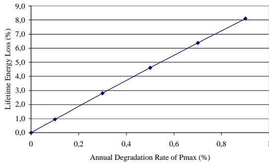
Fig. 7 The loss of Energy Life production as a function of annual degradation rates. Reports have placed this rate between 0.2% and 0.7% per annum [2, 4, 5, 6, 8]
