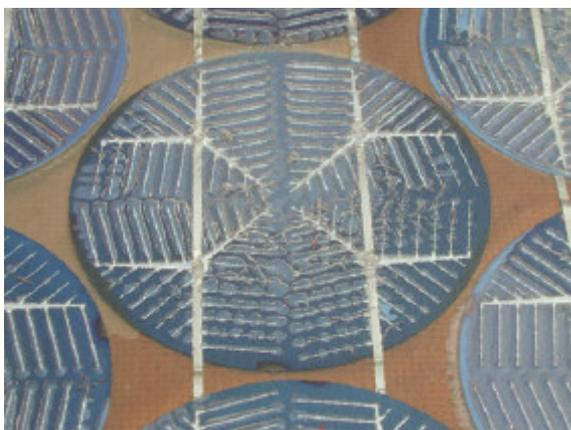
**Fig. 3** Example of severe discoloration and delamination.
