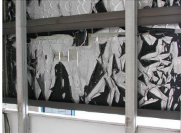
**Fig. 4** Splitting delamination of the back-sheet, note in this case the moisture ingress appears still to be blocked by the encapsulant.
