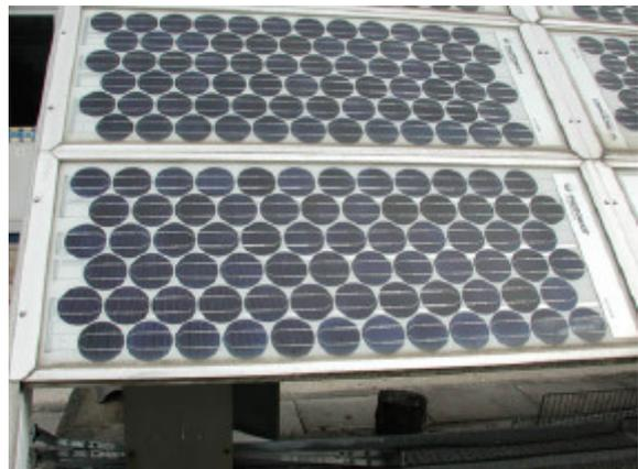
**Fig. 6** A set of 19 year old PV modules exposed at the JRC site which show none of the visible signs of degradation illustrated in Fig. 3 through 5.
