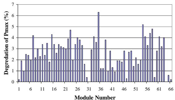
**Fig. 1** Summary of the degradation in P<sub>max</sub> after the Outdoor Exposure test for 66 module types tested at JRC Ispra.
