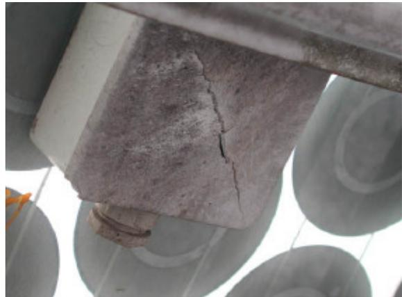
**Fig. 5** Junction box degradation leading to corrosion of the electrical connectors.
