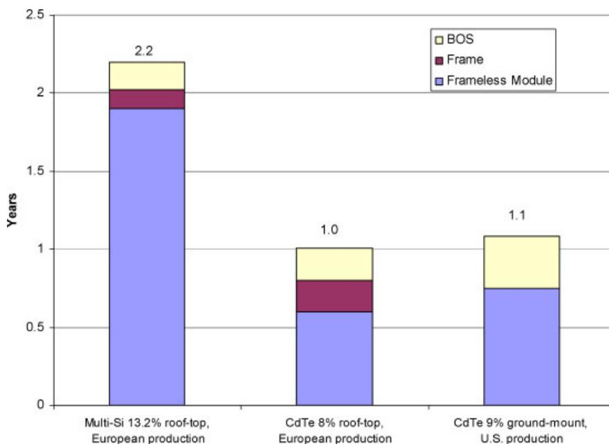
Figure 3. PV energy payback times of 2004 PV technologies for average southern Europe insolation ( $1700 \text{ kWh/m}^2/\text{yr}$ ), 75% performance ratio for roof-top installations, 80% performance ratio for utility ground-mount installations<sup>4-7</sup>
