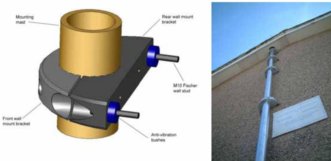
**Figure 4 - Correctly assembled & installed mast mounting brackets**
