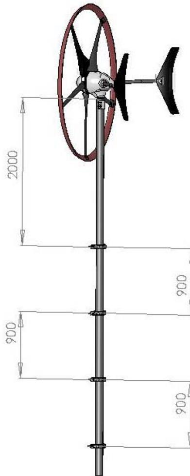
**Figure 5 - Swift™ wind turbine assembly showing bracket spacings**
