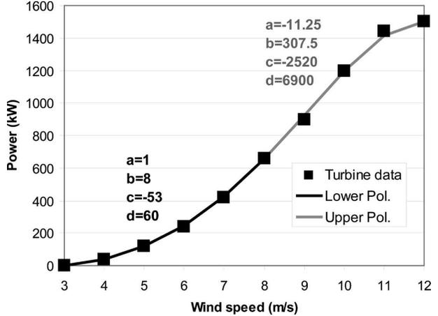
FIG. 1. Fitting curves for the GE 1.5-MW turbine.
